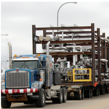
SAGD WELL PAD MODULES. BOTH MODULES COMBINED: 145' – 0" LONG X 16' – 0" WIDE
